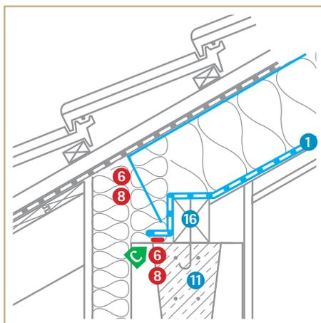
Knee wall sealing, sub-and-top with continuous rafter
