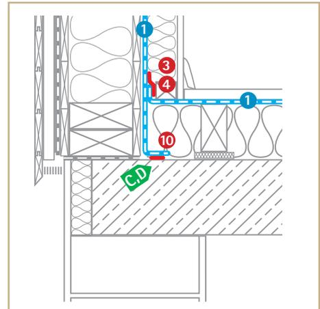
Sealing at reinforced concrete, ceiling or ground slab
