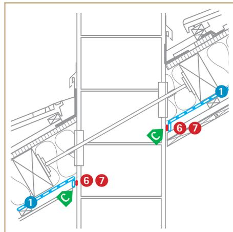
Sealing to plastered chimney
