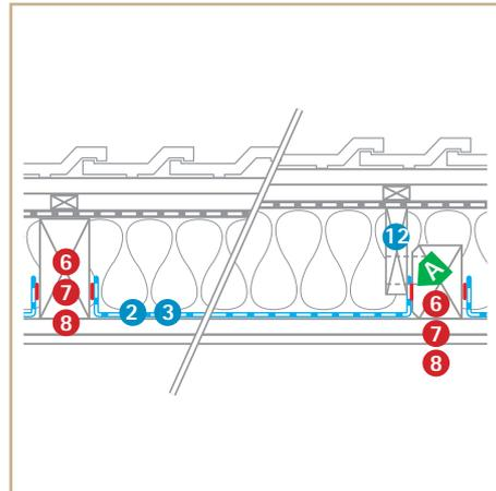
Vapour retarder, external installation, tub-shaped
