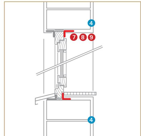
Sealing at windows, on the frame, masonry wall
