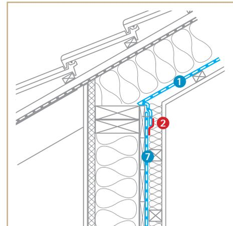
Sealing at knee wall for timber structures
