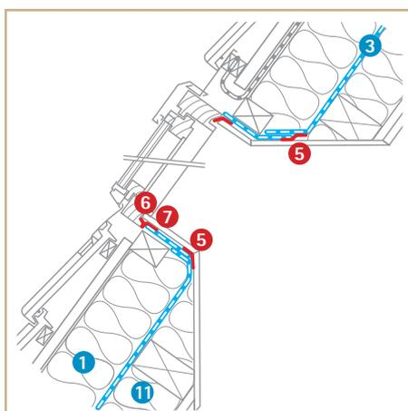
Sealing at skylights – Cross-section
