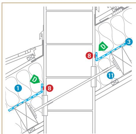
Sealing to plastered chimney
