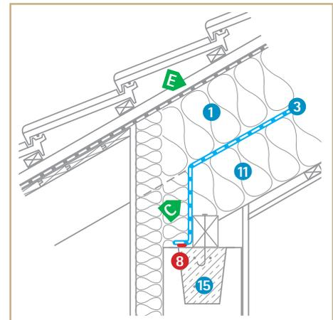
Sealing at knee wall with offset rafters
