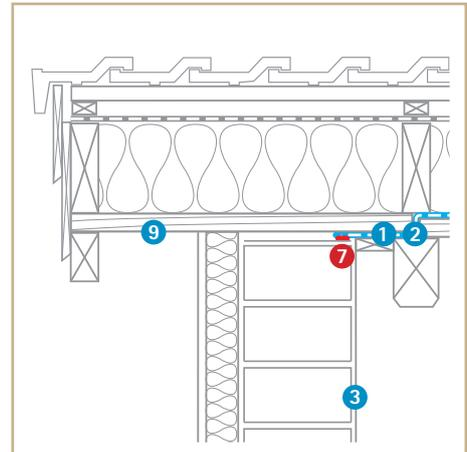
**Sealing at bargeboard with interruption at first visible rafter**
