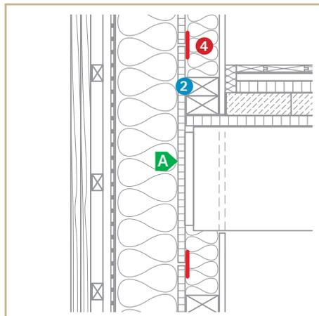
Sealing to beam, without penetration
