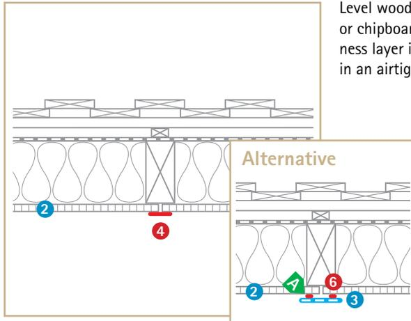
Level wood-based panels such as OSB, plywood or chipboard panels can be used as an airtightness layer if joints and connections are sealed in an airtight manner.
