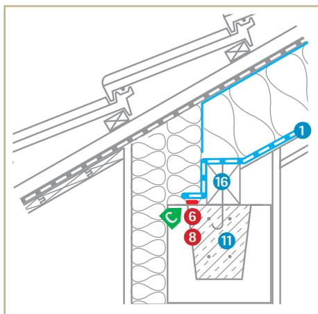
Knee wall sealing, sub-and-top with offset rafter
