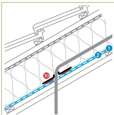
Cable feed-through for sub-and-top and tub-shaped
