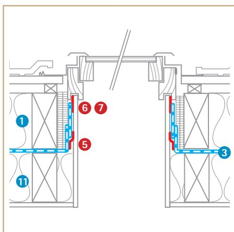
Sealing at skylights – Longitudinal section
