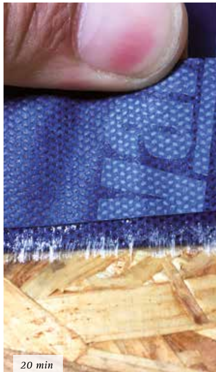
These photos show how strength builds up over the course of contact time. An adhesive tape was employed here that can be used for interior air sealing and exterior wind sealing. The initial adhesion – after 20 minutes – can be seen on the left; the significantly stronger adhesive bond after 24 hours can be seen on the right.
